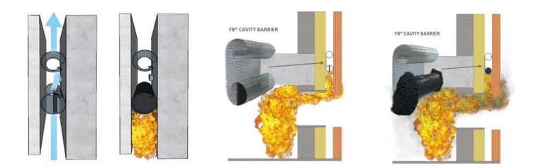
Just like fire compartments inside a building, **cavity fire compartments** prevent fire from entering or spreading to others.
